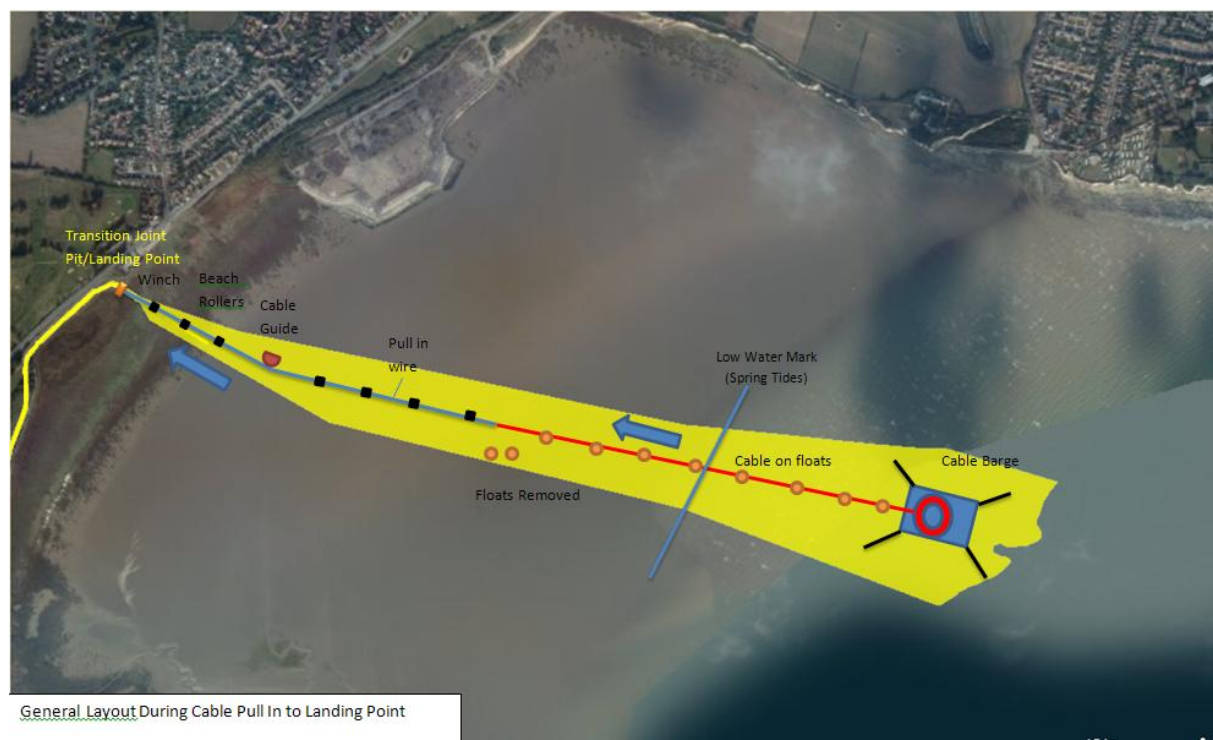
Figure 3. General layout during cable pull in across intertidal area.
