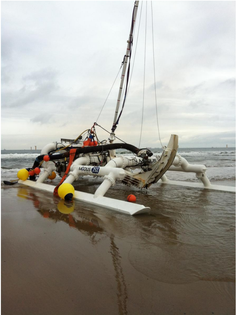
Figure 10. Cable Jetting Sledge
